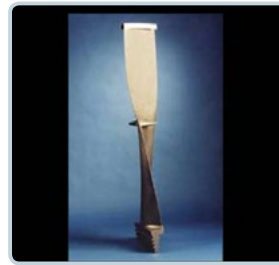
Compressor Blade Repaired by LENS System
