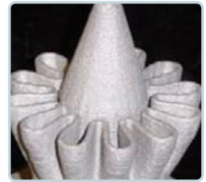
Exhaust Duct Fabricated by LENS System
