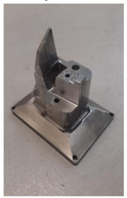
On the other hand, due to growing interest in Meltio technology from the tooling sector, we are currently developing processes for printing this interesting material combination, as you can see in the picture. We have developed geometries made in H11 with integrated cooling channels and inserts in CuCrZr.
